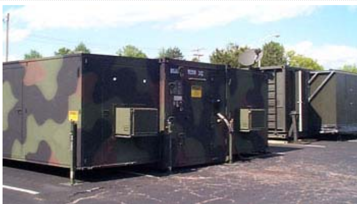
Focus: HOPE developed a "mobile parts hospital" (MPH) for the creation of spare parts and the repair of other parts at the military point of need.
