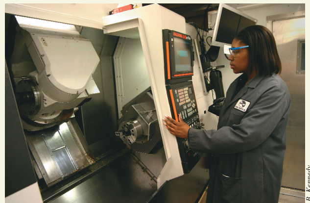
In a RMS currently being used for training at Focus: HOPE's Center for Advanced Technologies in Detroit, engineering candidate Shakemma Taylor works with the CNC of a Mazak multitasking lathe.
