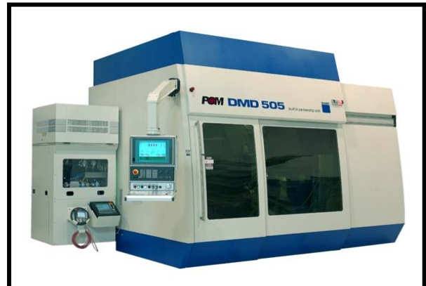
This POM Direct Metal Deposition (DMD) unit is one of the pieces of advanced manufacturing equipment that Candidates are exposed to in the Center for Advanced Technologies.
